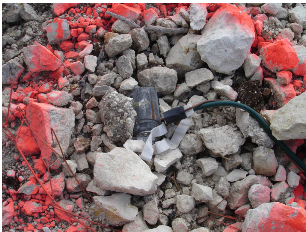
Figure 4. Positioning the MineBurner against a difficult target on a gravel bank. The 'memory' in the hose made the nozzle difficult to position (photo by the author).
