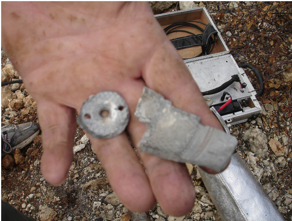
Figure 9. Three of the final five resulted in a deflagration, leaving large fragments and no evidence of a jet being formed (photo by the author).
