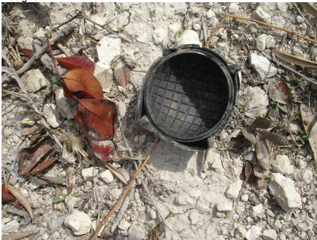
Figure 7. Results of the attack against the last intact BLU63. The two halves of the UXO were separated by six metres and the explosive burned out (photo by the author).
