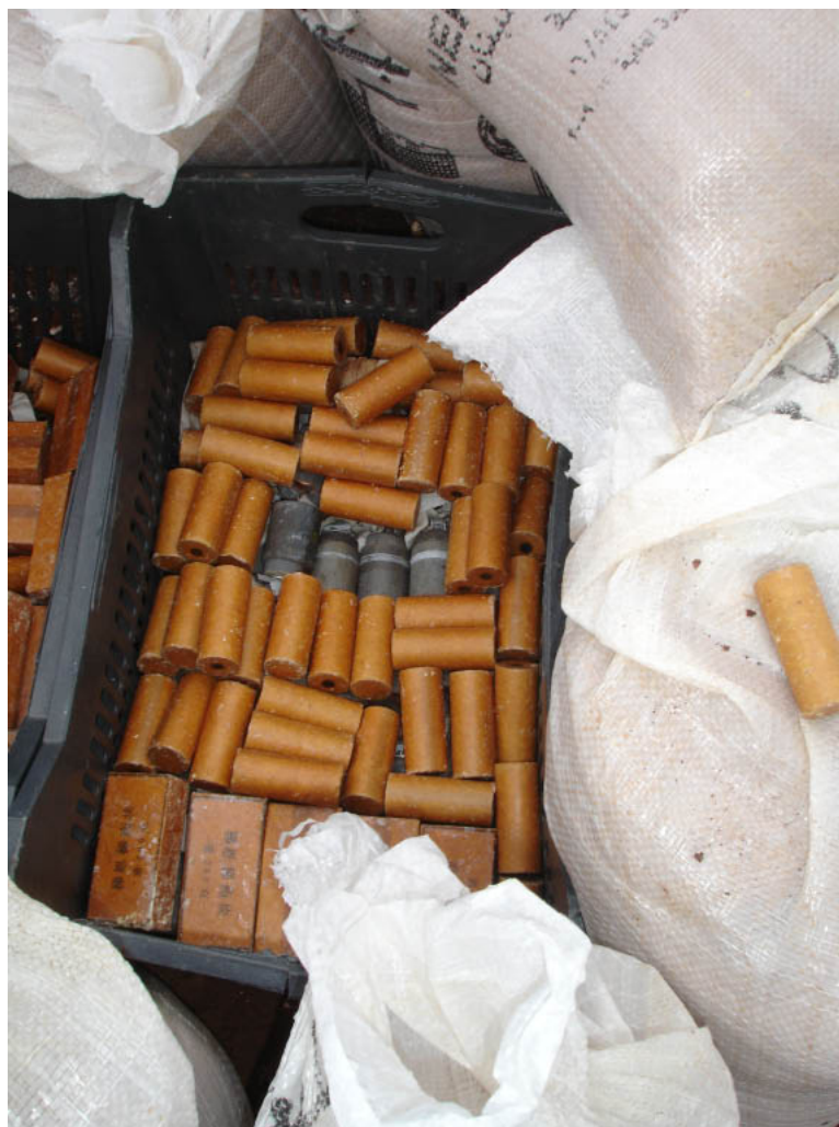
Figure 11. This multi-item demolition, being prepared by SRSA, shows the amount of high explosive that is required to demolish M42 targets (photo by the author).
