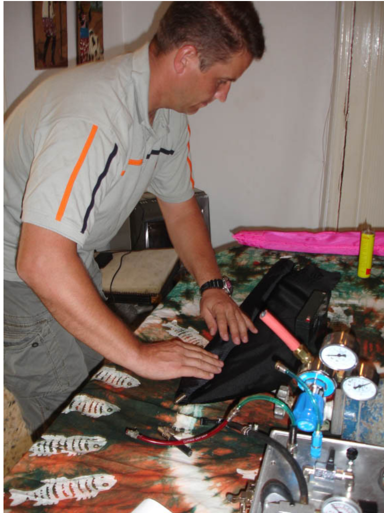
Figure 2. One of the NPA technicians learning to prepare a MineBurner (photo by the author).
