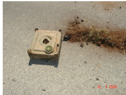
TMA-5 set up for burn
