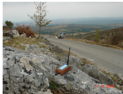
MineBurner set up showing repeater station
